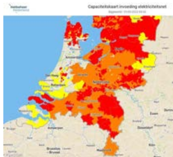
Source: Netbeheer Nederland, new installations cannot feed into the grid because of lacking network capacities – in red regions.
